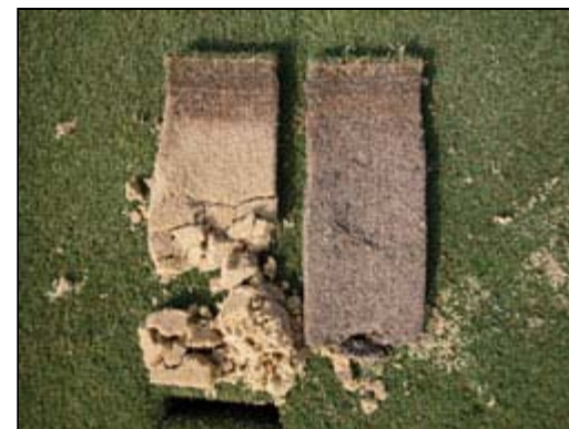
Image 1. Profile samples of nine-year-old rootzone plots visually indicate that very little organic matter has accumulated within the original rootzone (note yellow sand color of 100% sand profile on left) compared to the large amount of organic matter above the rootzone (note brown colored thatch-mat layer of both profile samples). Profile on right is from an 80:20 (v/v) sand-peat rootzone mix, which has a similar accumulation pattern.
